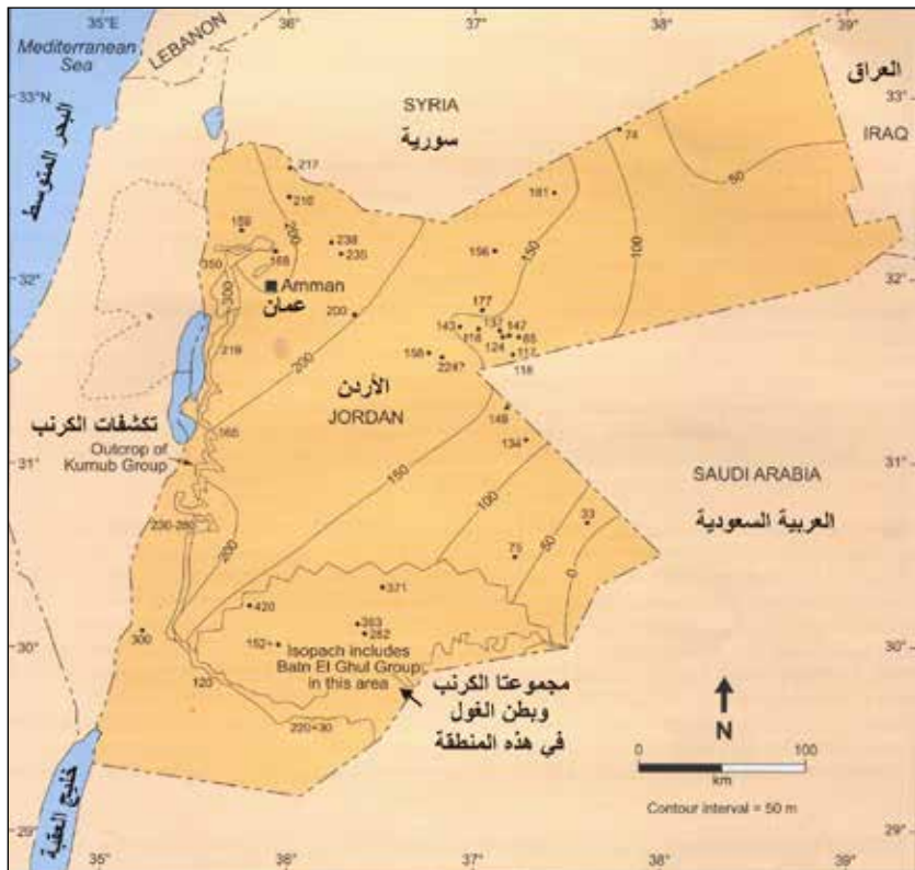
Figure 12 Distribution of thicknesses (isopach map) of the Kurnub Group throughout Jordan with the thicknesses in some borehole such as the Azraq basin (after Powell and Moh'd, 2011)
